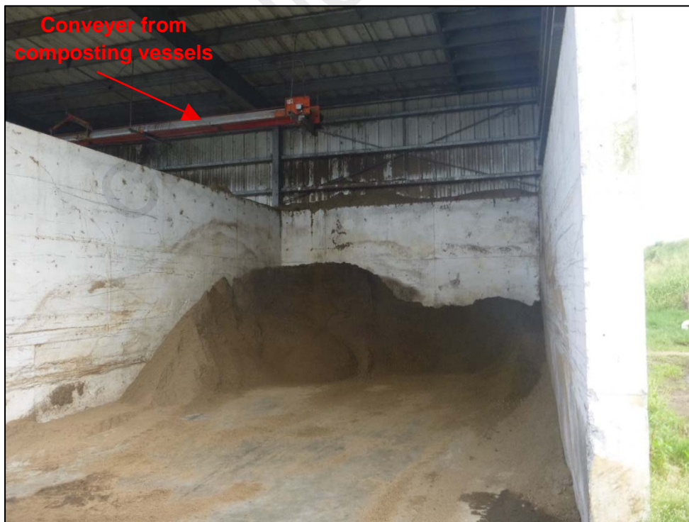
Photograph 18. A conveyor belt on the back end of the composting vessels conveys composted manure (i.e., cow bedding) into a covered stockpile stall. Photo by A. D'Angelo; 12/14/16.
